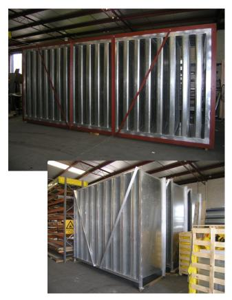
**GCS** Acoustics Rectangular Silencers are used to reduce noise levels within air paths such as Air-conditioning ducting fan extraction systems. Commonly they are used within plant rooms to silencer the internal noise to the outside surroundings.
